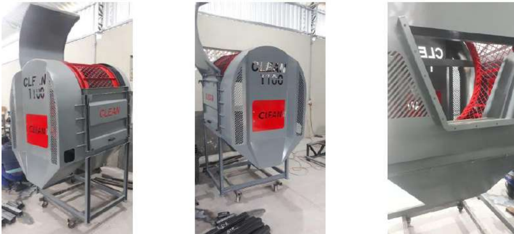
Figure 8 – Peneira rotativa do forno Clean
