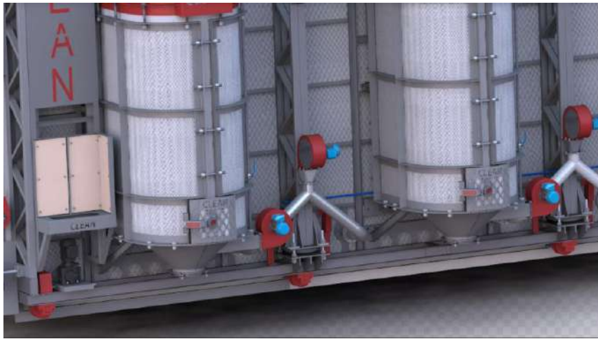
Figure 10 - Air injection system for combustion of biomass
